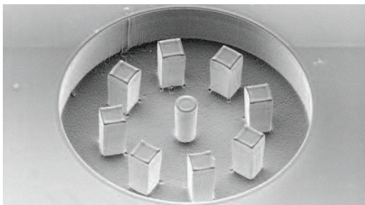
Micromachined Si supports on underside of PZT membrane
